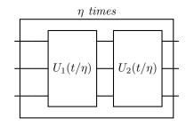
2. The block encoding formalism has been shown recently to allow for Hamiltonian simulation with less ressources compared to the Trotter approach. While the optimal scenario is based on "quantum signal processing" (QSP), we will use here as illustration a less optimal method known as linear combination of unitaries (LCU).
